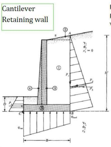
Rankine's active pressure acting on AB; Rankine's pasive pressure acting on the vertical line at the toe;
