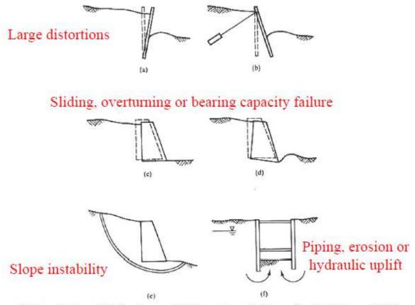
Figure 2-2 Mechanisms of failure of retaining walls (Atkinson, 1993)
