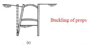
Figure 2-3 Structural failures of retaining walls (Atkinson, 1993)
