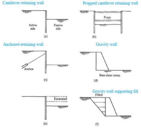
Figure 2-1 Principle types of retaining structure (Atkinson, 1993)
